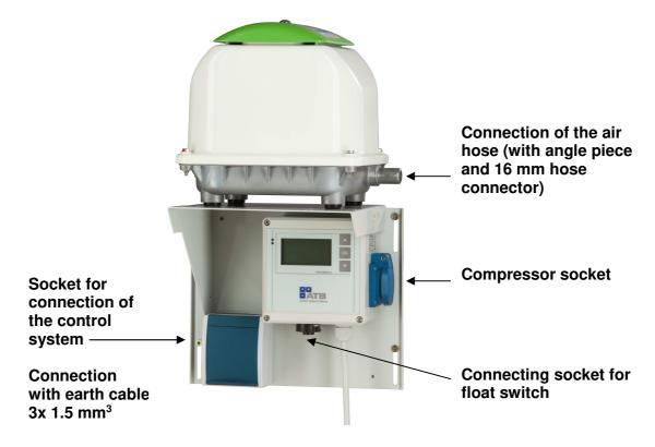
Install the control unit either directly to the console on a stable wall or in the cabinet which can be supplied as accessory (inside cabinet/open air column). The maximum separation between tank and mounting location of the control unit may not exceed 10 m.
