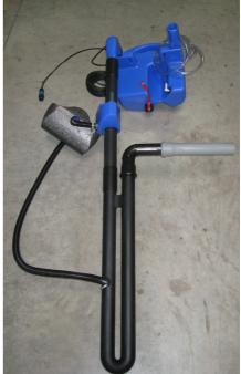
Determine the position of the float bracket on the air lift pump: the bracket is so secured for height (diag. right), that the upper edge lies 5 cm below the outlet (see page 9).
