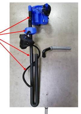
As standard, a connecting pipe is inserted through the dividing wall, onto the parts of the overflow baffle are plugged (for details on mounting the overflow baffle, see page 10). The connection pipe of the overflow baffle must be removed first.
