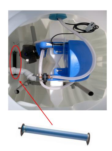
With the 10 EW variant, a 1070 mm long tube aerator is positioned on the tank bottom in the longitudinal direction of the tank (marking on the right). Enlarged spacers are mounted on this tube diffuser to prevent the membrane for the contact with the tank bottom.
