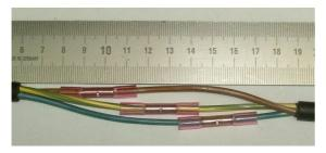
7. Crimp the butt connectors **only** with a crimping tool. Choose the correct jaws according to the colour of the cables, in this case red. Please check the result after crimping by pulling the cables easily. The crimping process ist done correctly when the cables can't be pulled out of the butt connectors and when the insulation of the butt connectors isn't damaged.
