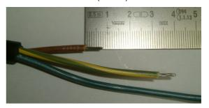
5. Crop the shrink hose with scissors in suitable length. After shrinking the hose has to be 5 cm over the outer cover of the cable on the right and on the left side. Drag the cropped shrink hose onto the cleaned cable.
